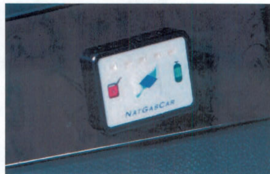
Two fuel rails and two sets of fuel injectors feed the same port in the intake. The computer starts the car on petrol, and then switches to gas when the engine is warm. The indicator button below is the only clue that this car runs gas.
